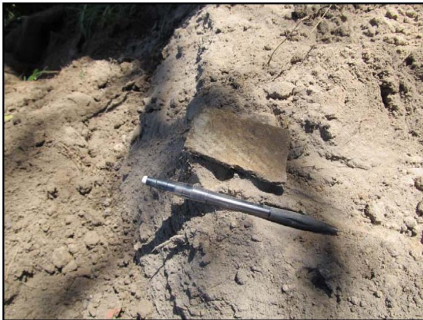
Photo 4: Photograph of ACM fragment in TP4 , Lot 422.
