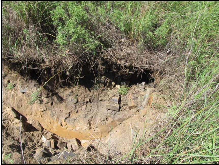
Photo 3: Photograph showing Fill profile in TP2 on Lot 422 with refractory brick in sandy matrix.
